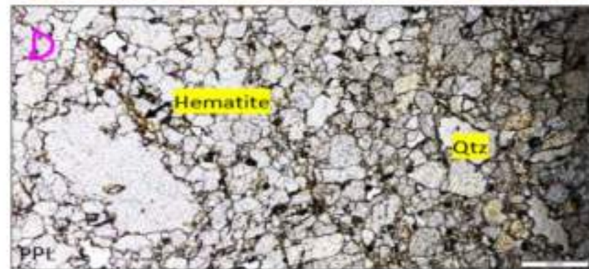
Figure 5: A and B shows a thin section of quartzite both in XPL and PPL at scale of 200µm whereas C and D is at a scale of 1mm.
