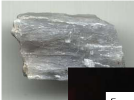
Petalite - Lithium Aluminium Phyllosilicate \text{LiAlSi}_4\text{O}_{10} (Contains around 4.8% \text{Li}_2\text{O} )
